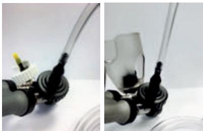
With a bottle mount tubing combination it is recommended to partially prime the tubing side first, than afterwards the bottle mount side. This will avoid product waste on the bottle mount side during the priming of the tubing.
